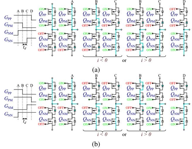
Fig. 4: Voltage polarity based bidirectional commutation cell commutation process for: (a)  $v > 0$  (-ve mid-point voltage-edge), and (b)  $v < 0$  (+ve mid-point voltage-edge).
