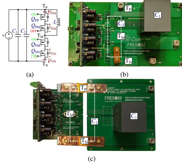
Fig. 8: (a) Double pulse test setup ( $L = 93.5 \mu\text{H}$ ,  $C_1 = 25 \mu\text{F}$ ,  $C_2 = 4 \times 100 \text{ nF}$ ), (b) Back-to-back TO-247-4 package SiC MOSFETs based half-bridge PCB, and (c) BiDFET half-bridge module PCB. Dotted lines indicate commutation loop.
