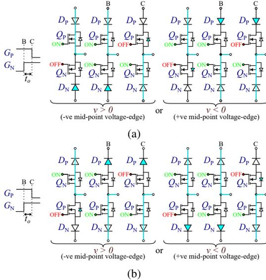
Fig. 3: Voltage-bidirectional commutation cell commutation process for: (a)  $i > 0$ , and (b)  $i < 0$ .
