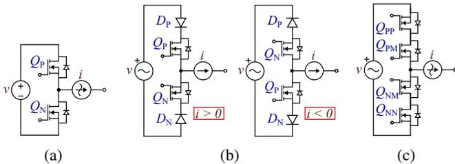
Fig. 1: Types of commutation cells: (a) current-bidirectional, (b) voltage-bidirectional, and (c) bidirectional.
