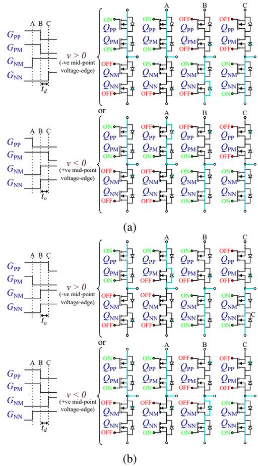
Fig. 6: Voltage and current polarities based bidirectional commutation cell commutation process for: (a)  $i > 0$ , and (b)  $i < 0$ .
