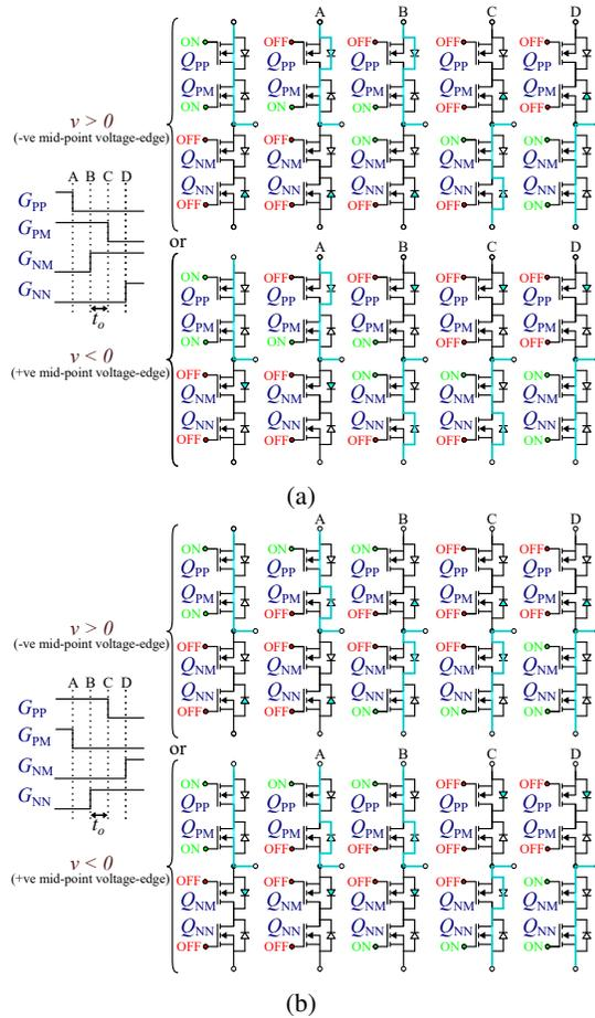
Fig. 5: Current polarity based bidirectional commutation cell commutation process for: (a)  $i > 0$ , and (b)  $i < 0$ .
