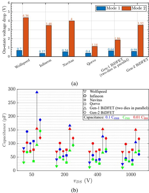
Fig. 7: (a) FQS on-state voltage drop at 20 A, and (b) FQS constituent FET capacitances variation with  $v_{DS}$ .
