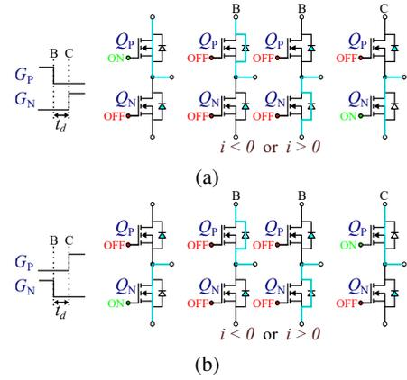
Fig. 2: Current-bidirectional commutation cell commutation process for: (a) -ve mid-point voltage-edge, (b) +ve mid-point voltage-edge.
