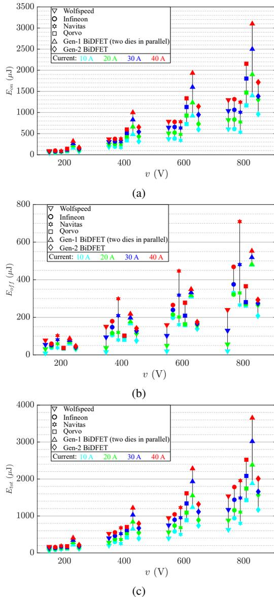
Fig. 10: Switching energy variation with voltage and current at 25 °C: (a) Hard turn-on ( $E_{on}$ ), (b) Hard turn-off ( $E_{off}$ ), and (c) Total ( $E_{total}$ ).
