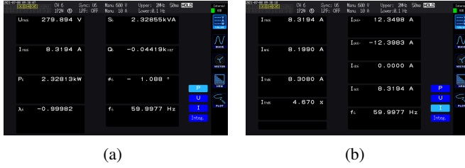
Fig. 8: (a) Power factor and (b) current THD at 100% load.
