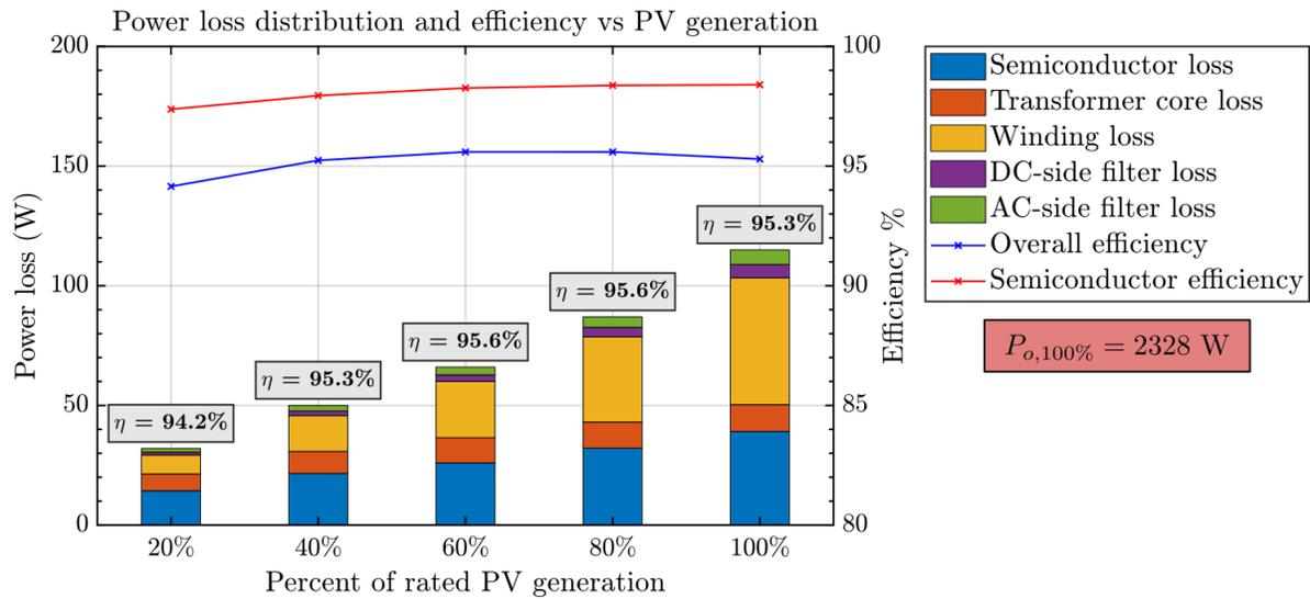
**FIG 5 Single-phase ac-dc converter overall efficiency, semiconductor efficiency and estimated loss distribution at different rates of PV generation.**
