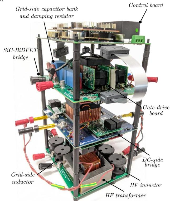
**FIG 3 Hardware prototype of the 2.3 kW, 400 V to 277 V<sub>RMS</sub> single-phase AC/DC DAB converter using Gen-1 BiDFET enabled matrix converter on ac side.**
