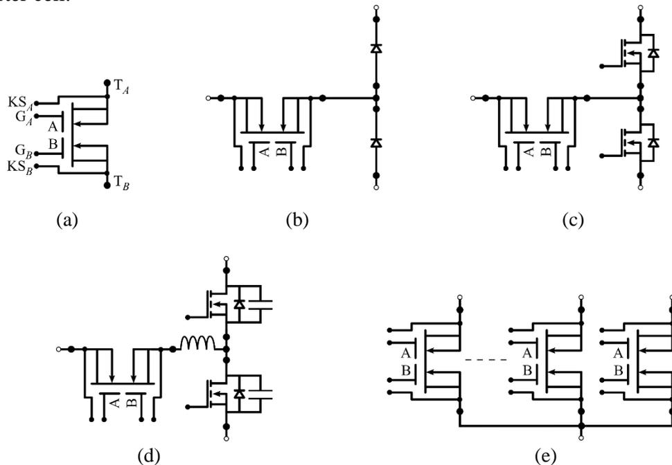
**FIG 1 (a) BiDFET symbol:  $T_A$  and  $T_B$  are source terminals,  $G_A$  and  $G_B$  are gate terminals,  $KS_A$  and  $KS_B$  are kelvin source terminals, and arrows denote body diodes of the constituent JBSFETs, (b) Current-injection type converter cell, (c) T-type converter cell, (d) Resonant type converter cell, (e) Matrix type converter cell.**
